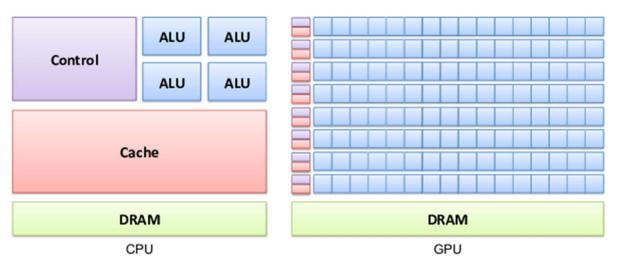
Figure 4: The Parallel Processing Architecture of a GPU Enables Faster Computation Than a CPU That Enable a Wide Number of AI Applications
